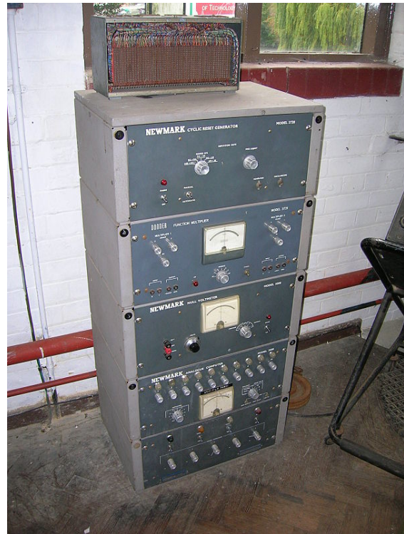
A 1960 Newmark analogue computer, made up of five units. This computer was used to solve differential equations and is currently housed at the Cambridge Museum of Technology.
