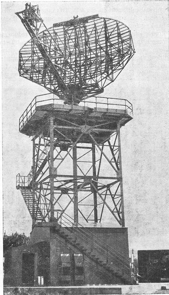
Fig. 4 — 23 cm Radar S654 — example of modern 'L' band equipment with twin horn aerial feed
