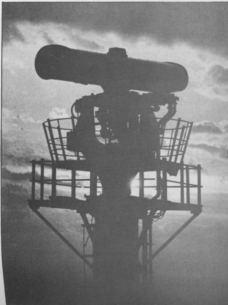
3 High-performance dual frequency naval surveillance radar
