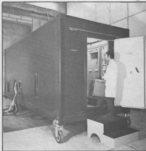
9 Martello transmitter container in environmental test chamber
