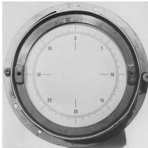
Figure 18. Sketch of the circular CRT display used by Klein Heidelberg [5] and the actual LB13/40 tube (Bauer [31]). The same display tube was used in the WÜRZBURG radar, where the 0 – 40 scale corresponded to range in km.
