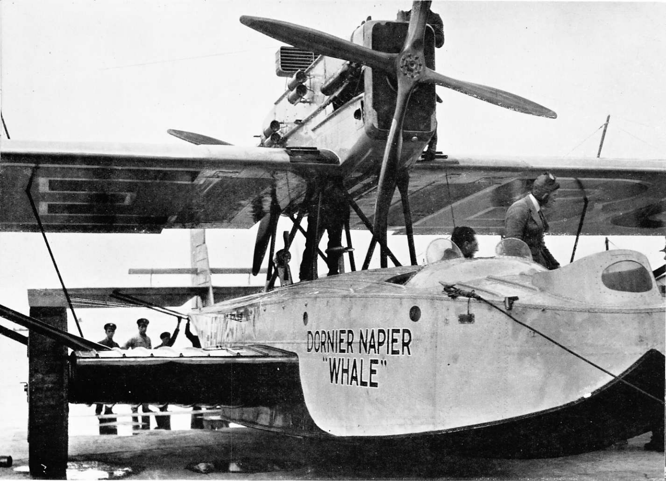
Captain Courtney's machine. In flight a 200 ft trailing aerial was used; on the water a 40 ft telescopic mast. For the Marconi Bellini Tosi direction finder fixed loop aeriels were fitted from wing-tip to wing-tip and from bow to stern
