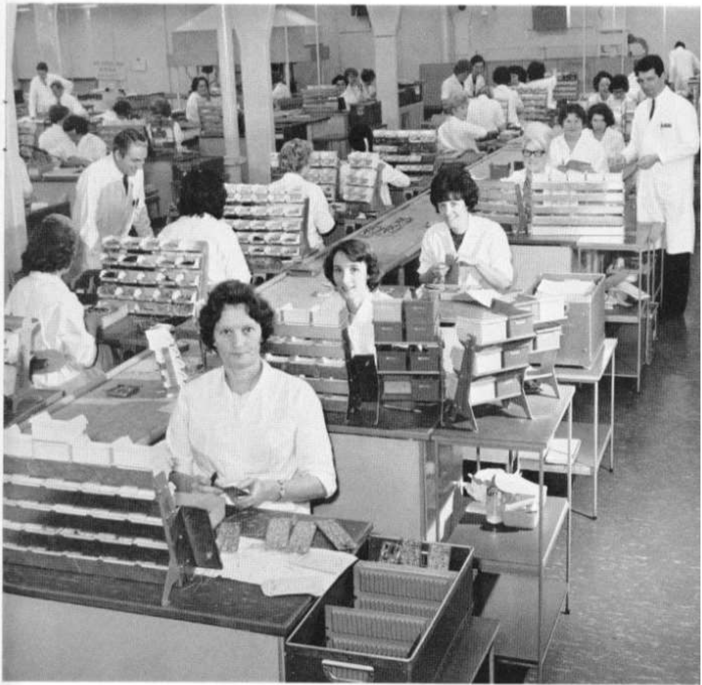
Assembly on the production line before the boards go for flow soldering. Standing are chargehands Alf Kimber, left, and Jim Jewell
