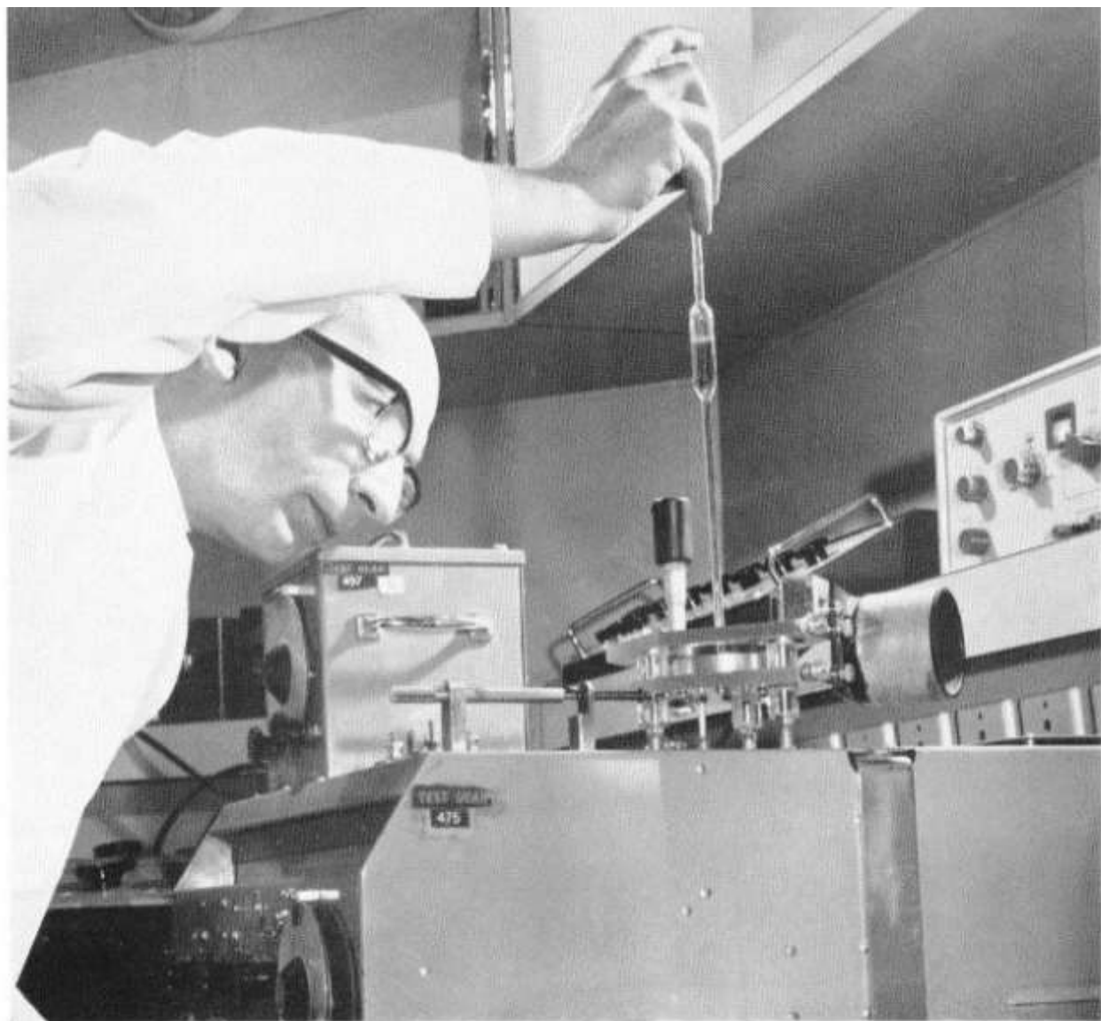
Filling the liquid jig before making dielectric measurements on oil. Ken Sheed, standards engineer, uses the M.I. TF 70AC dielectric loss test jig
