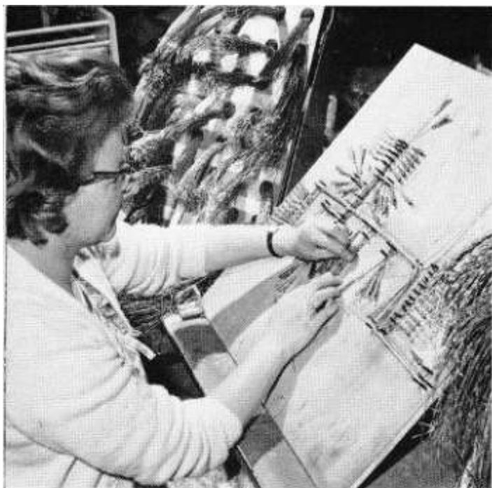
LEFT: Mrs. Betty Mortlock making the colourful cableform which goes right round the voltmeter. She finds the special holder, made to contain the pre-cut wire, most useful. RIGHT: The power unit being assembled by Susanta Basu and the sub-assemblies being put together by Geoff Merrett, who also attaches the probes
