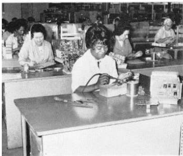
These pictures show the new layout of the benches and supply racks. ABOVE: Circuits being assembled for H2000 MST communications receivers, which are being sold all over the world, some to NATO. The girls position the components by the numbers on the plan and tack them in with solder. Left to right, Mrs. Doxie James, from Jamaica, Gwen Cox and Mrs. Ruby Freeman. BELOW, LEFT: Mrs. Hazel Bailey, centre, who also operates the flow-soldering machine which completes the joints. To the left, behind, is Mrs. VI Rees, and right, Mrs. Irene Blake. BELOW, RIGHT: Mrs. Cora Porteous at work on H2000 circuits
