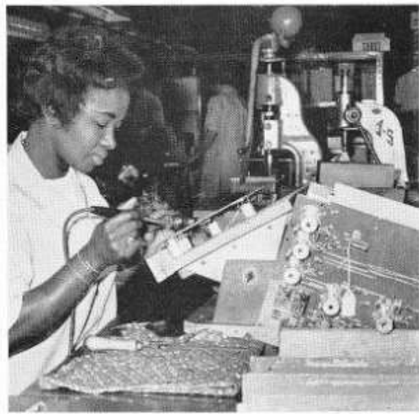
These pictures show the new layout of the benches and supply racks. ABOVE: Circuits being assembled for H2000 MST communications receivers, which are being sold all over the world, some to NATO. The girls position the components by the numbers on the plan and tack them in with solder. Left to right, Mrs. Doxie James, from Jamaica, Gwen Cox and Mrs. Ruby Freeman. BELOW, LEFT: Mrs. Hazel Bailey, centre, who also operates the flow-soldering machine which completes the joints. To the left, behind, is Mrs. VI Rees, and right, Mrs. Irene Blake. BELOW, RIGHT: Mrs. Cora Porteous at work on H2000 circuits
