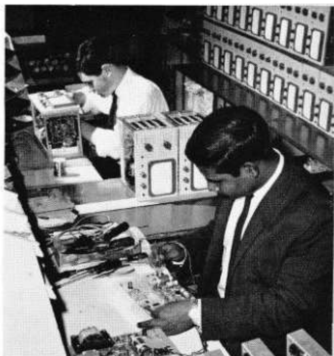
LEFT: Mrs. Betty Mortlock making the colourful cableform which goes right round the voltmeter. She finds the special holder, made to contain the pre-cut wire, most useful. RIGHT: The power unit being assembled by Susanta Basu and the sub-assemblies being put together by Geoff Merrett, who also attaches the probes
