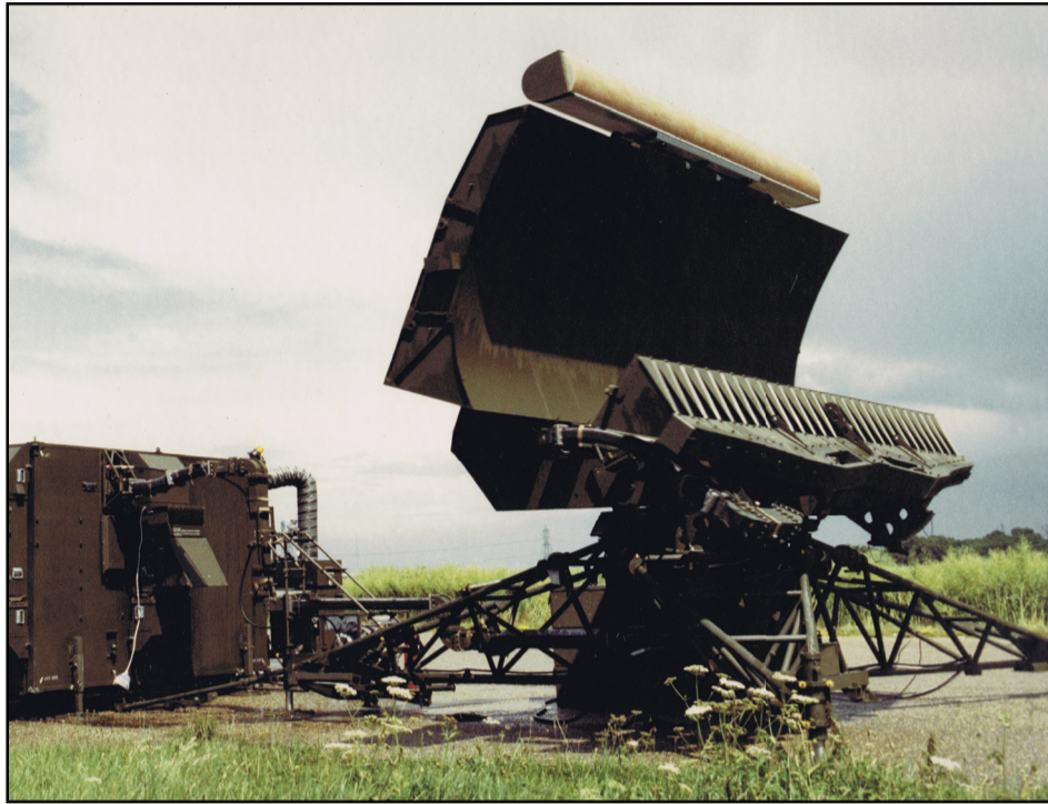
A S600 Radar deployed along with its control cabin and mobile power supply. This gives the Radar the ability to operate in the field at remote sites. (NEDAD.2013.146)
