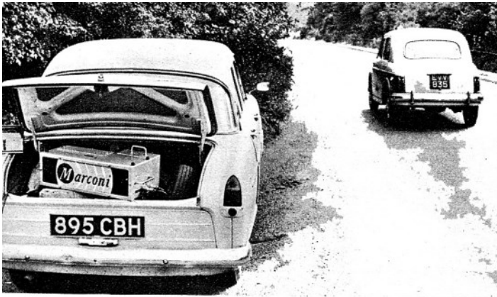
Deliberate wrong alignment of the aerial to send the beam straight down the road can increase readings by up to 3 m.p.h. at 50 m.p.h.; for accuracy the oblong box with the Marconi sign should be at right angles to the kerb
