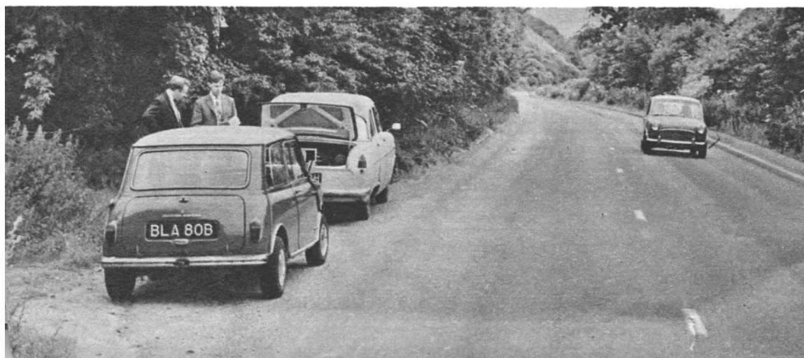
Driver's eye view of a typical setup, showing how even a Mini can obscure a police trap, with the aerial unit in the boot of the Consul; there must always be at least one observer near enough to the aerial to be able to look along the path of the radar beam.
