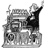
Deliberate wrong alignment of the aerial to send the beam straight down the road can increase readings by up to 3 m.p.h. at 50 m.p.h.; for accuracy the oblong box with the Marconi sign should be at right angles to the kerb
