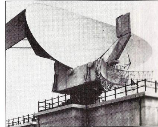
Figure B3. Large horizontal dimension gives beamwidth under half-degree because of short wavelength (10cm).
