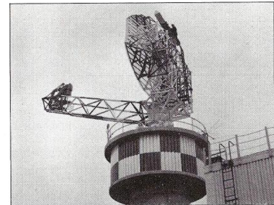
Figure L4. L-band (23cm) air traffic control radar S654 of the RCAF.
