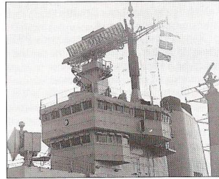
Figure E1. Note the difference in size of the tracker, surveillance and navigational radars on HMS Invincible. (Nav. radar just above right hand end of surveillance.)
