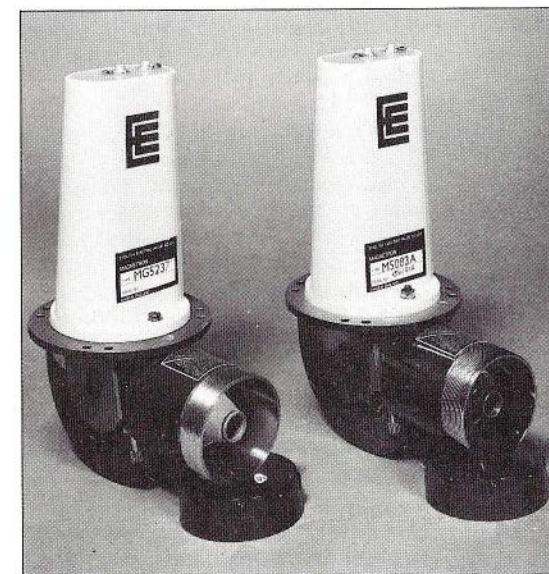
Figure M3. Modern high efficiency, tunable magnetrons made by English Electric Valve Co. for the Marconi airfield surveillance radar Type S511. It generates a peak pulse power of 600 kilowatts at a wavelength of 10 cms (two versions shown).
