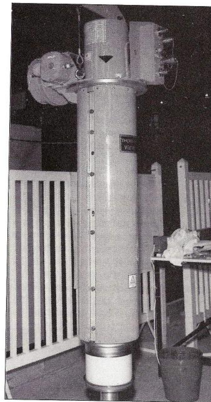
Figure K1. L-band (23cm) hybrid amplifier (Twystron), used in Martello S713 with a peak power output of 3.3 MW
