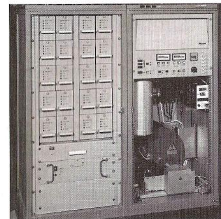
Figure T1. Modern transmitter with TWT and modular modulator.
