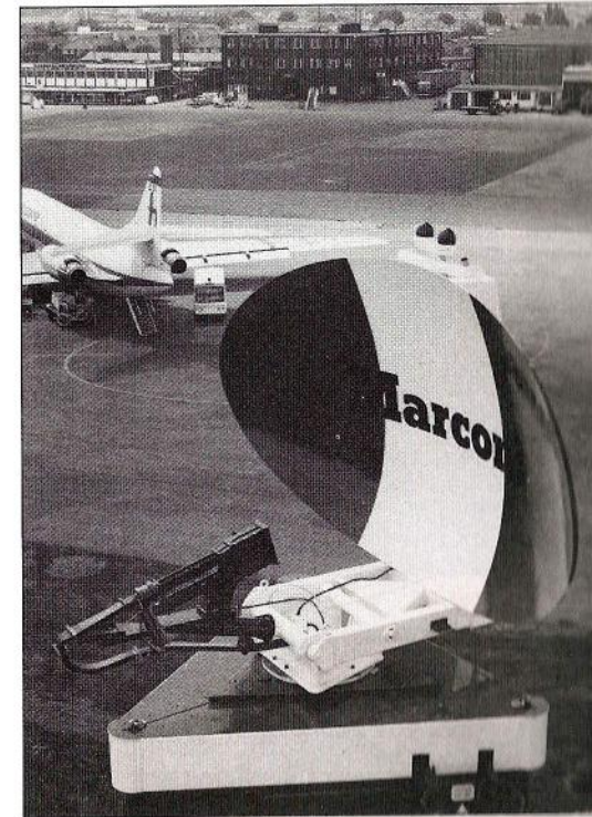
Figure A3. Martello planar array of 2560 elements (23cm wavelength).
