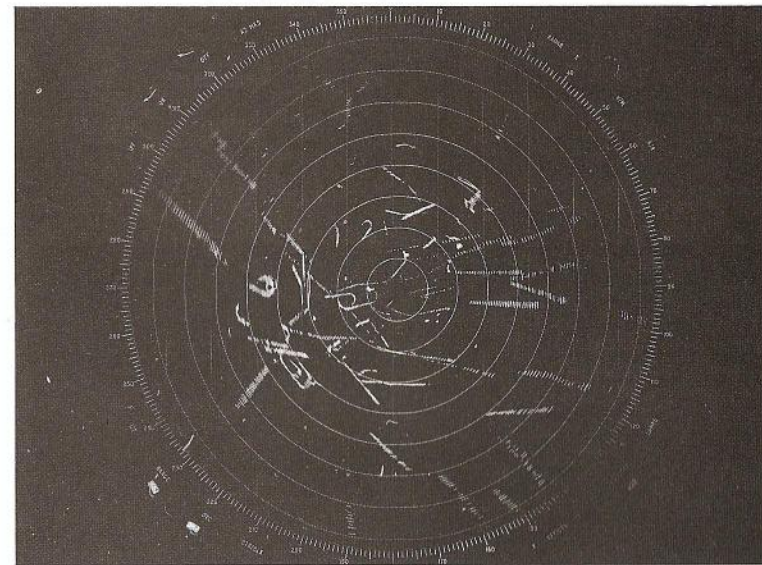
Figure C2 Processed radar display, with clutter removed.
