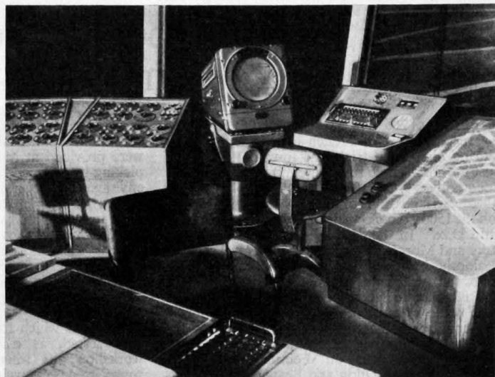
Fig. 5—Part of the air traffic control room at London Airport showing the surface movement radar display unit. The mimic diagram desk on the right is a separate equipment
