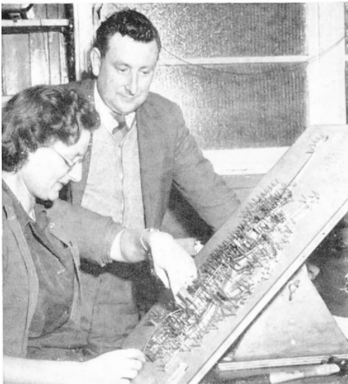
In the Cableform Section Sid Steele, charge-hand, watches Mrs. Doreen Staines while she makes a cableform for a Mark IV camera control panel
