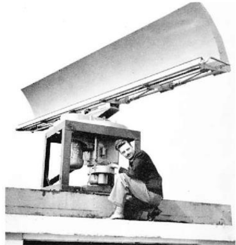
The aerial of the SNW50 storm detection radar when on test at Rivenhall. This particular equipment has now been installed at the new Salisbury Airport in Rhodesia. With the aerial is Colin Downs who has been working with Eric Royle of Radar Division
