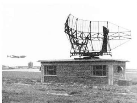
Our radar at London Airport. This is the aerial of the S.232 used for the control of aircraft leaving the London area. It is an all-weather equipment and will work in heavy rain. The Television O.B. van used in the demonstration was parked near this radar
