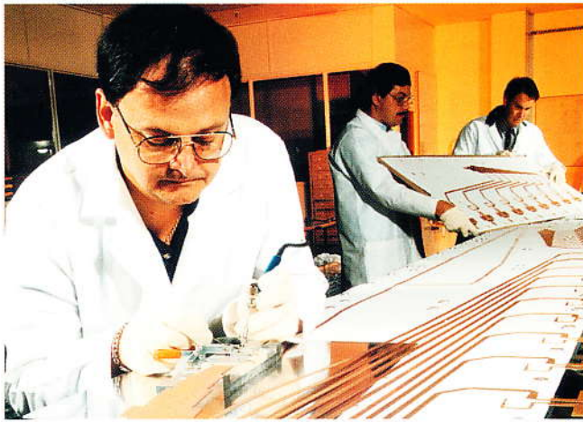
Precision cut antenna assembly
