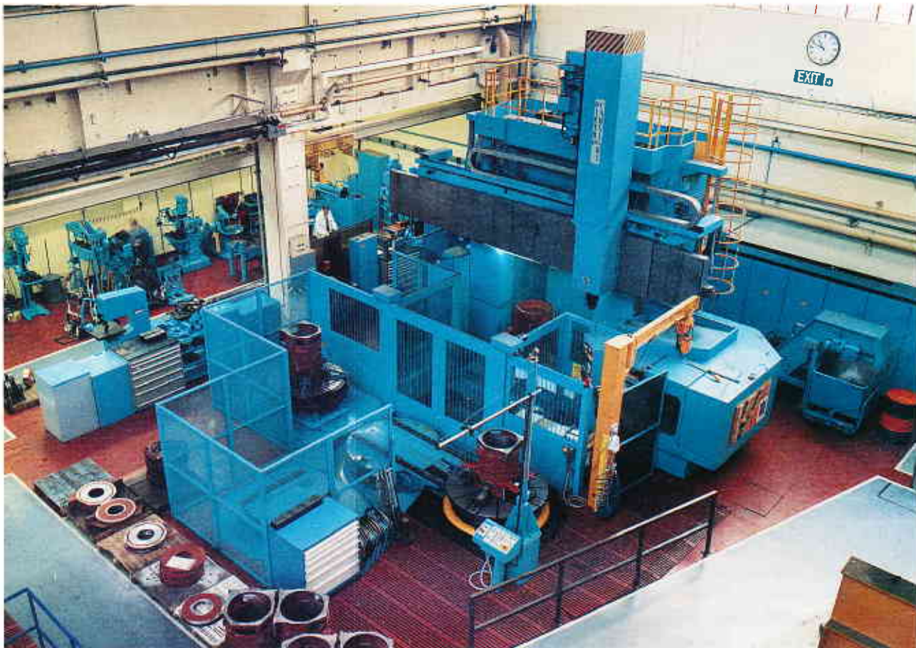
9 Two metre cube, 7-axis machining centre
