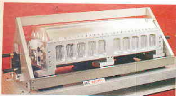
23 Breadboard laser with stable resonator mount
