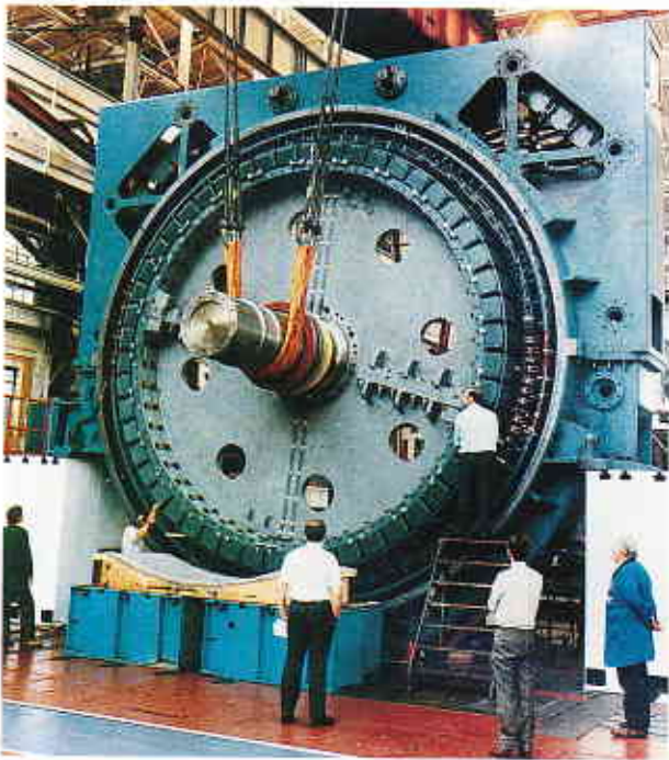
18 The 44MW synchronous propulsion motor capable of powering the Q.E.2 at 32 knots
