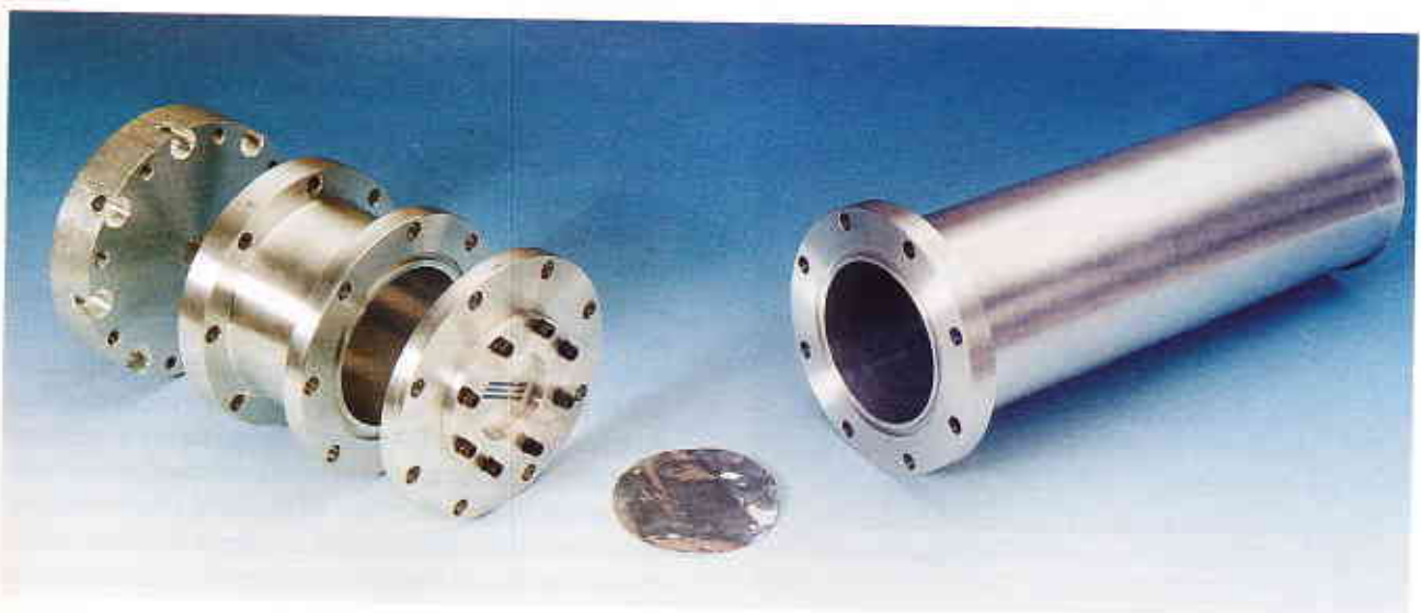
15 The Applied Physics Division's laser pressure pulse simulator
