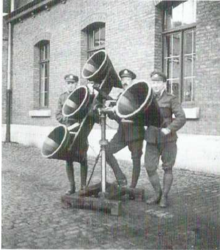
Figure 10. Transportable WW1 sound locator
