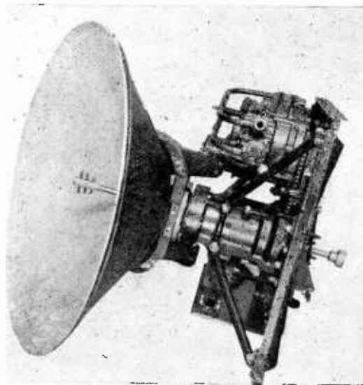
Mechanism for spiral scanning with a single paraboloid reflector in the centimetre-wave AI equipment.
