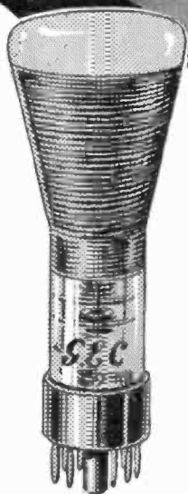
A typical G.E.C. Cathode Ray Tube 4102, with 2 1/2" screen, widely used in industry during the war, and with many peacetime applications.
