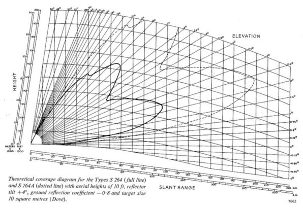
THESE multi-purpose surveillance radar sets are developed from the well known and well proved Marconi Radar Type S 232, offering similar facilities, with improved performance.
