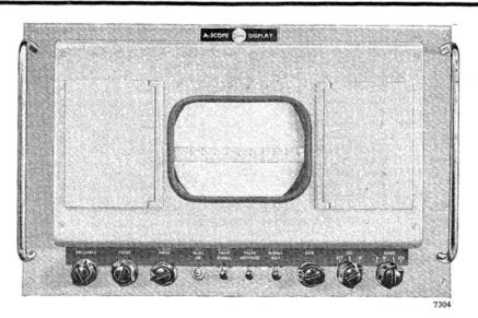
THE DISPLAY UNIT TYPE SD 600 is an 'A' – scope of compact construction, using a 6-in. diameter display tube with a ground and polished flat face.
