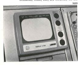
front panel. Provision is made for fitting an edge-illuminated graticule for use where a pre-determined format is to be used.
