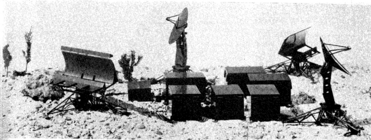
S 600 sophisticated high capacity radar system with two plan radars on different frequency bands, with Multiple transmitters in diversity, two heightfinders with transmitter in frequency diversity, secondary surveillance radar, and a powerful data handling and display complex based on the MYRIAD computer
