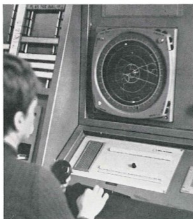
11in. S3006 Direct View Storage Tube Display in operation at Ostend Airport
