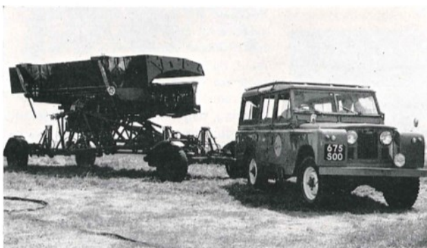
The 10cm (S) Band surveillance aerial ready for towing
