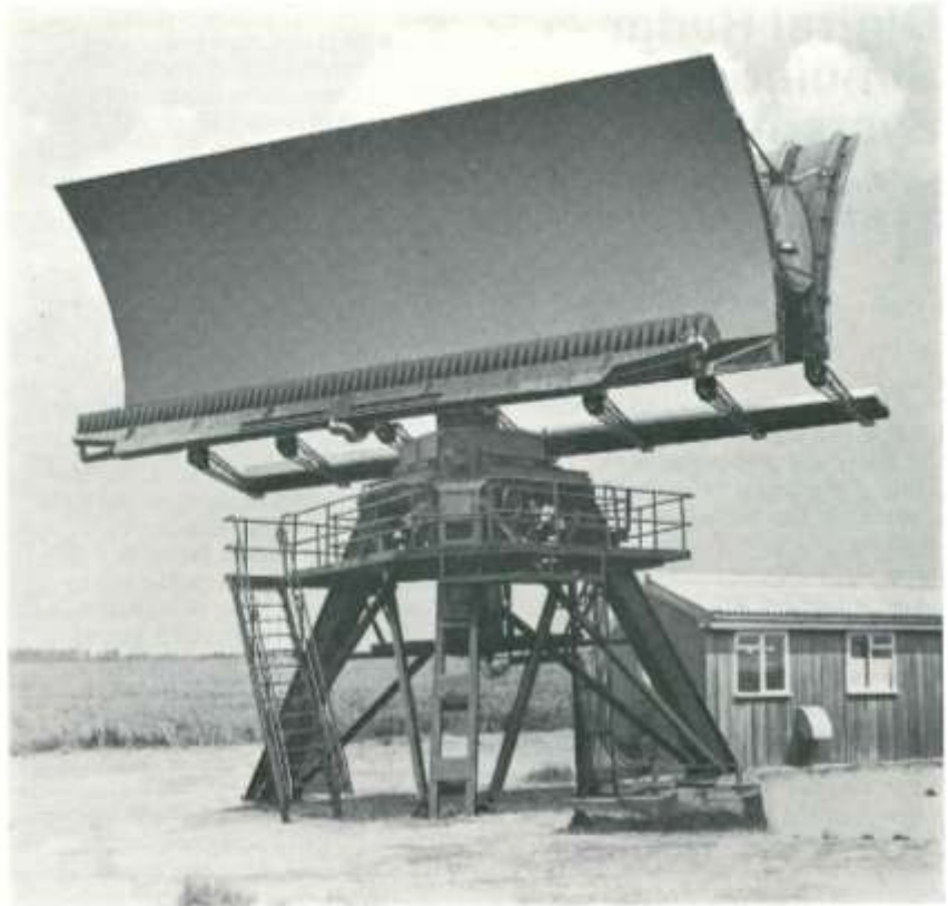
10cm (S) Band and 23cm (L) Band static back-to-back surveillance radar S631
