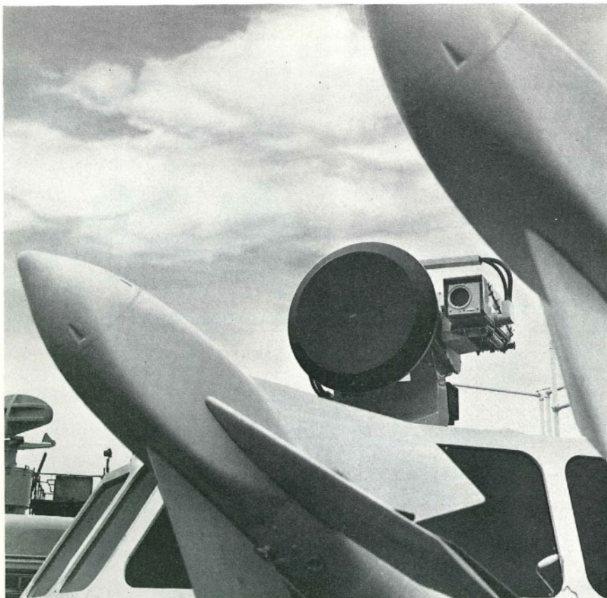
The ST 801 lightweight tracking radar
