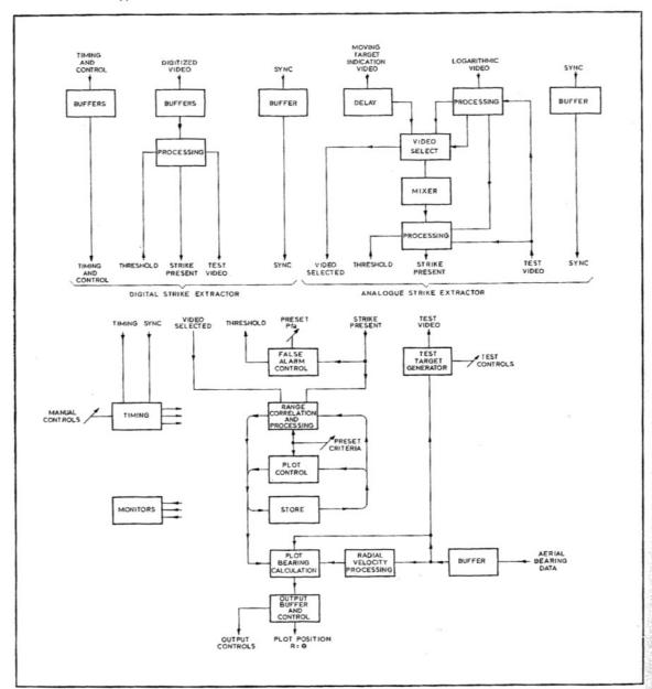
Block diagram for the Primary Radar Plot Extractor Type S7200
