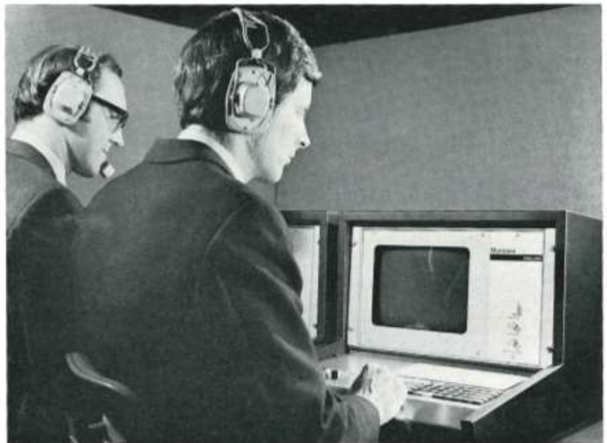
Two trainees at simulated pilots' positions in an S600 radar simulator system
