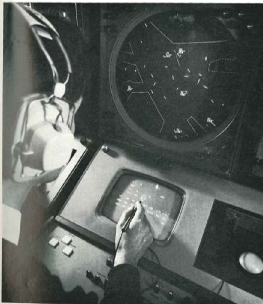
A synthetic radar display with selection being controlled through tabular display and light pen
