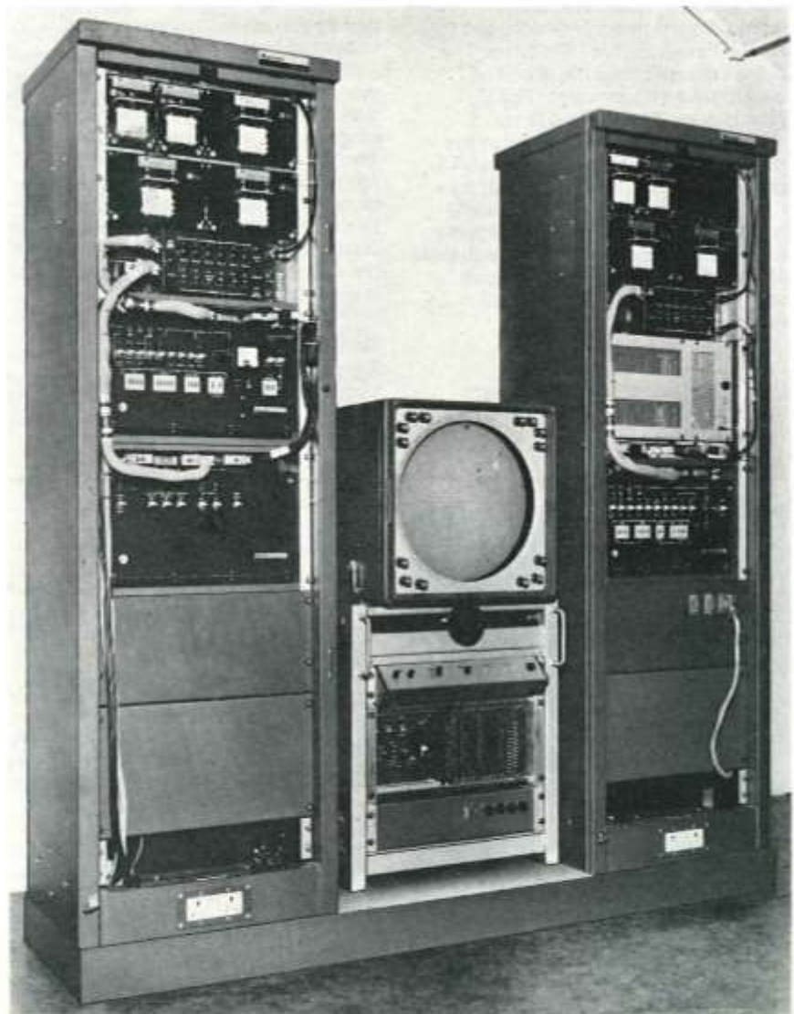
Primary and secondary plot extraction and monitor display system
