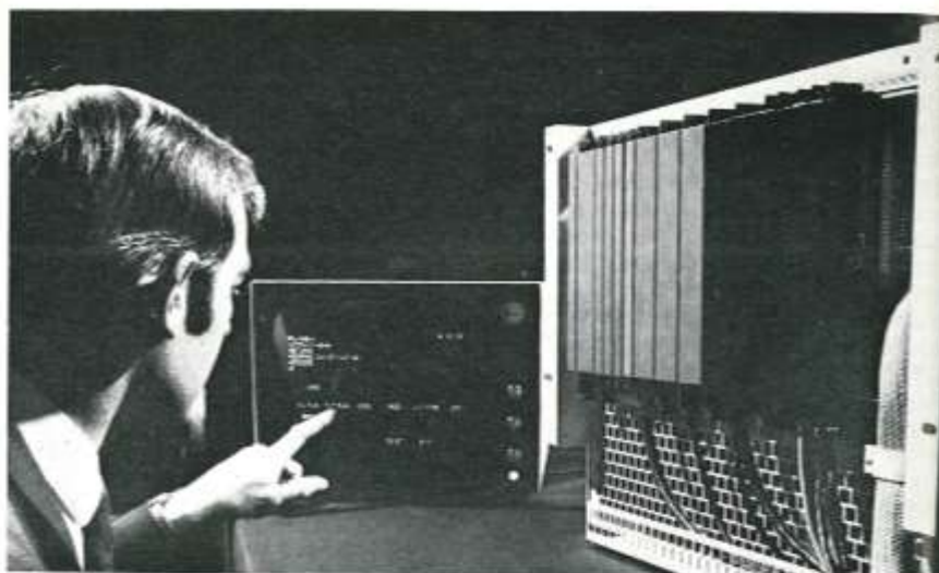
A processing bin from the Locus 16 series, with touch-wire display in the background
